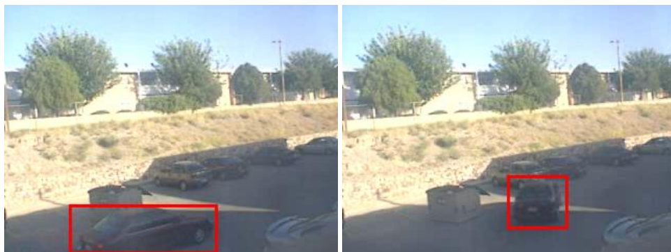
Fig. 3. A bounding box indicates the location of an object in motion.
