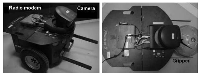
**Figure 1. The robotic soccer player. A lateral view (left) and a superior view (right).**
