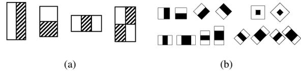
Figure 1. (a) Haar features introduced by [21]. (b) Extension to the basic set proposed by [11]
