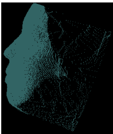
Fig. 11. Snapshot of the constructed three dimensional model without any triangle and texture.
