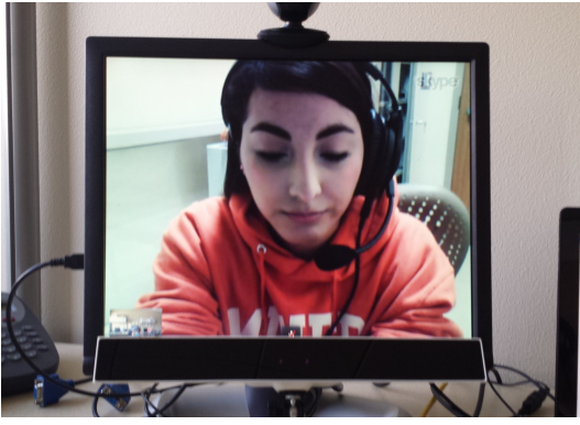
Figure 1: Participant’s view, with webcam above and gaze tracker below the screen.
