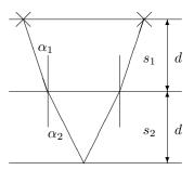
In particular, we can thus determine the paths from the source to each sensor. The travel-time  $t_i$  along i-th path can then be determined as the sum of travel-times in different cells j through which this path passes:  $t_i = \sum_j \frac{\ell_{ij}}{v_j}$ , where
