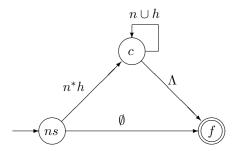
Now, all that remains to do is to go from here to the 2-state a-automaton by eliminating the remaining state c:
