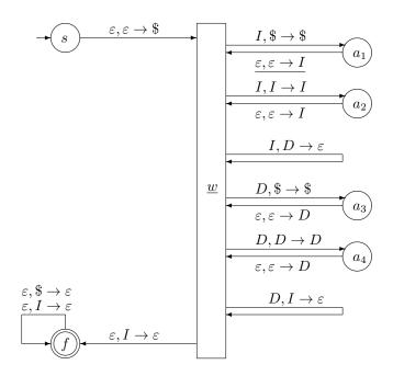
After that, we read the last symbol I. Since I is on top of the stack, we first go to  $a_2$ , then push I into the stack and go back to the working state.
