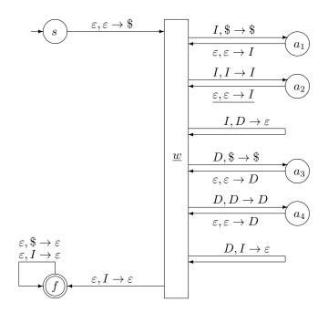
We have read all the symbols, so we move to the final state; in that move, we pop the top I from the stack, so the stack only contains one I on top of the dollar sign:
