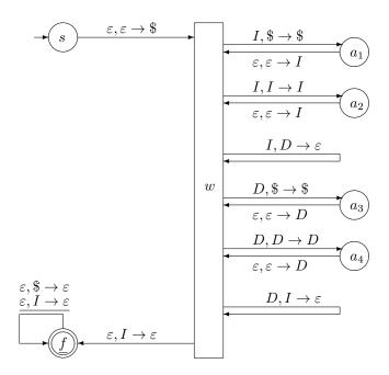
Finally, we pop the dollar sign from the stack, so we are now in the final state with an empty stack, so the word is accepted.
