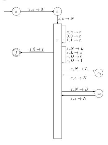
The stack is now empty. We are in the final state with the empty stack, so the word a01 is accepted.
