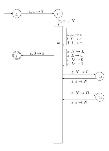
The only thing we can do when in the state s is push the dollar sign into the stack and get to the intermediate state i:
